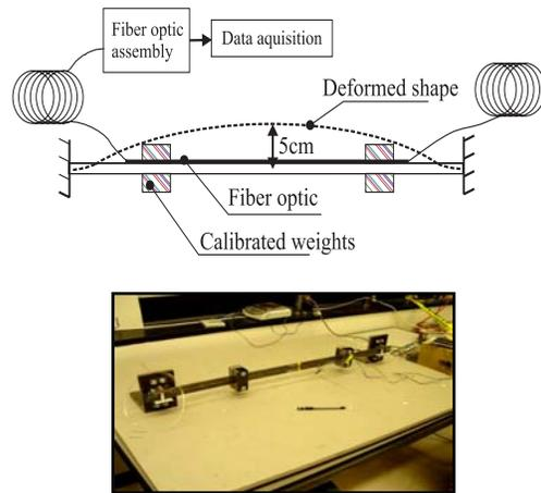
Figure 7. Oscillation test set-up
